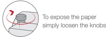
To expose the paper simply loosen the knobs
